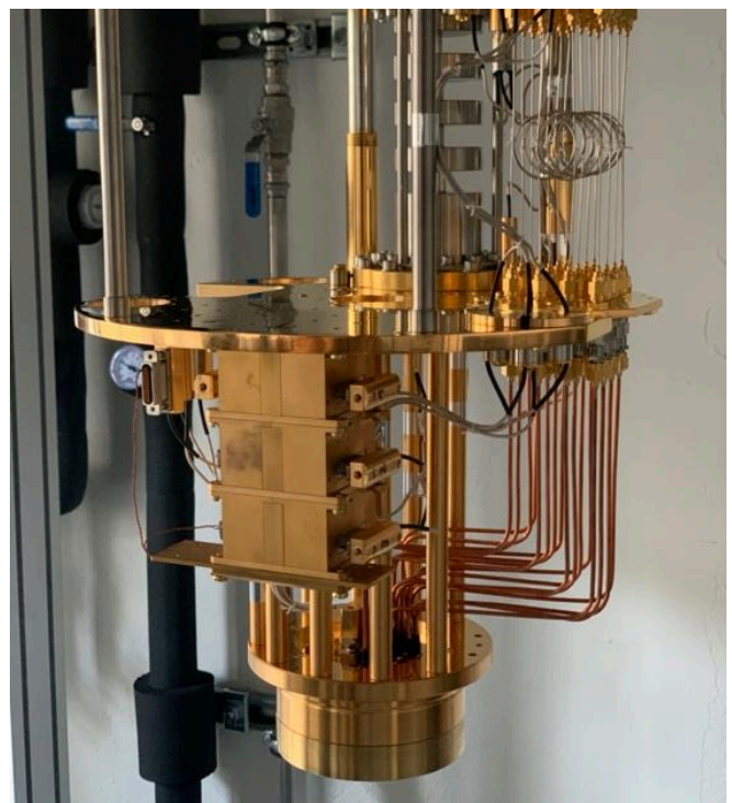
Three stacked MFT filter boxes under test in a dilution fridge at Uni Basel.
